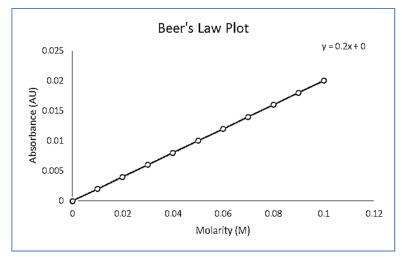
A is the absorbance of a solution being measured by the colorimeter  $\epsilon$  is a proportionality constant called the molar absorptivity b is the path length of the cuvette, usually 1cm c is the molarity of the solution
