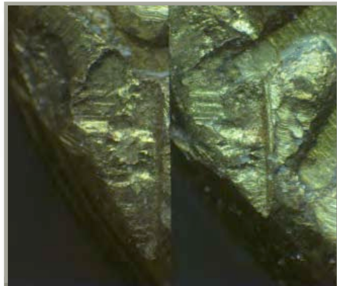
Microscopic comparison of ejector impressions on two cartridge cases.
