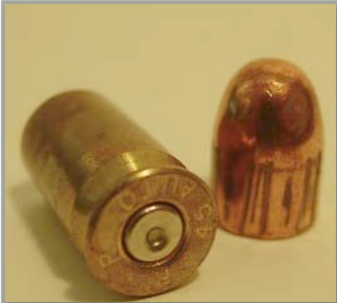
A fired cartridge case and a fired bullet. Note the firing pin impression on the primer of the cartridge case and the land and groove engraving on the bullet.
