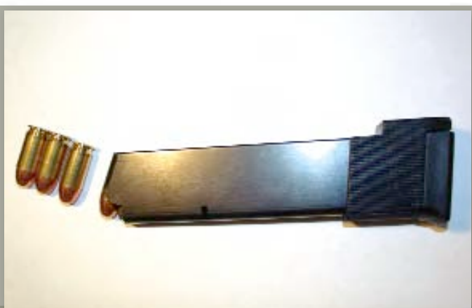
The side view of an ammunition magazine with the orientation of the cartridges that are to be inserted.
