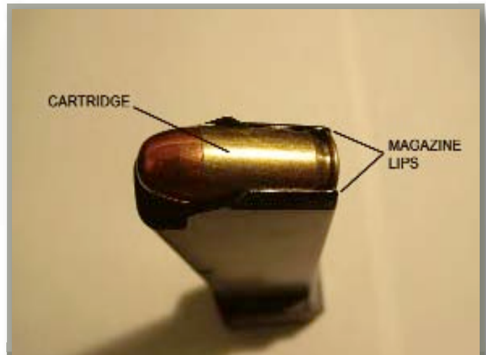
A cartridge in an ammunition magazine. The top cartridge held in place by the two magazine lips.
